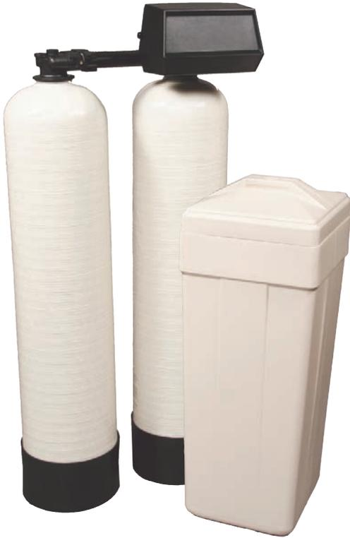
Hard water passes through the online media tank that contains resin beads coated with sodium ions. The calcium and magnesium ions are exchanged for sodium (or potassium) ions, thus softening the water. When the beads have trapped the hardness and need to be regenerated, the 9100 control valve charges them with the brine from the brine tank.
